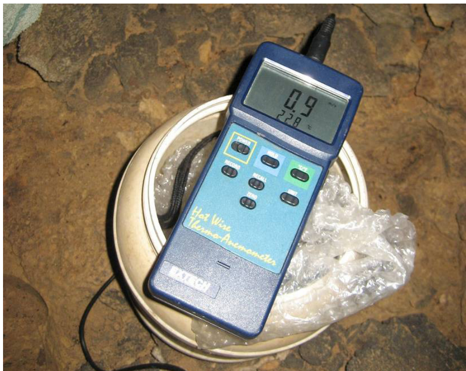
ExTech Hot Wire Thermo-Anemometer reading in the Africa passage
