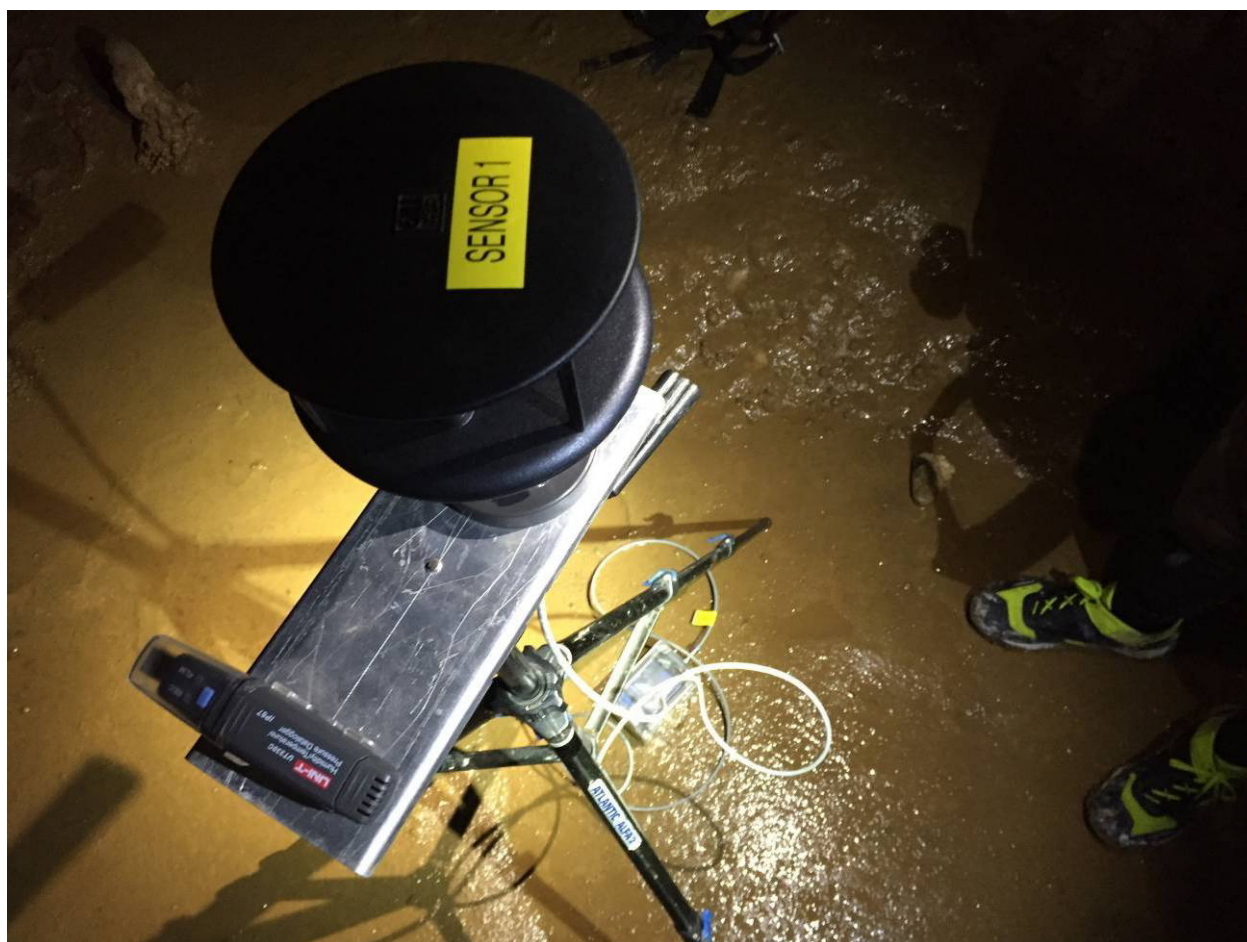
Typical arrangement: Windsonic anemometer, aligned to north, mounted on a lightweight plate and tripod and connected to the W10 Spacelogger via a 3m cable. The UNI-T330C Datalogger is on the mounting plate beside the anemometer and is held in a clip.
